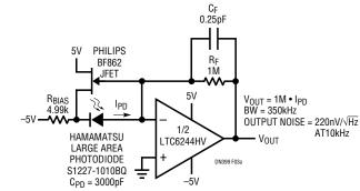
Figure 3a. Large Area Diode Bootstrapping
