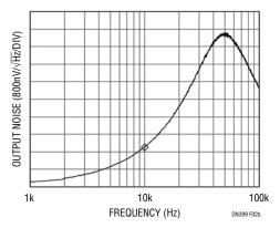
Figure 2b. Output Noise Spectral Density of the Circuit of Figure 2a. At 10kHz, the 1800nV/ $\sqrt{Hz}$  Output Noise is Due Almost Entirely to the 7.8nV Voltage Noise of the LTC6244 and the High Noise Gain of the 1M Feedback Resistor Looking into the High Photodiode Capacitance
